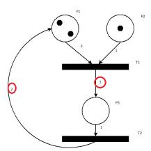
The effect matrix (E) has a p number of rows (each for each place in the system) and t columns (each for each transition in the net). It is defined as the difference between the output matrix and the input matrix.
